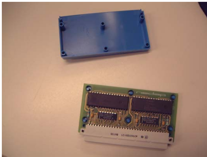
Figure 3: Insides of a Ballot Module
